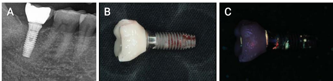
Figure 2. Failed implants cases with no fluorescence. A: Radiograph obtained just before the implant fell out. There was no peri-implant bone loss, B: Removed implant structures (White-light image), C: Removed implant structures (Fluorescence image).
